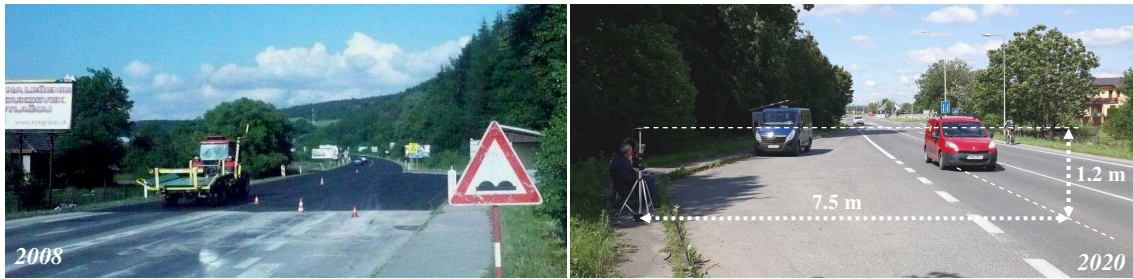
Figure 2. Views of the measuring station on the BUS stop by the road I/61 in Dolný Hričov on 8.6.2008 and 23.6.2020 with an indication of measuring distances.
