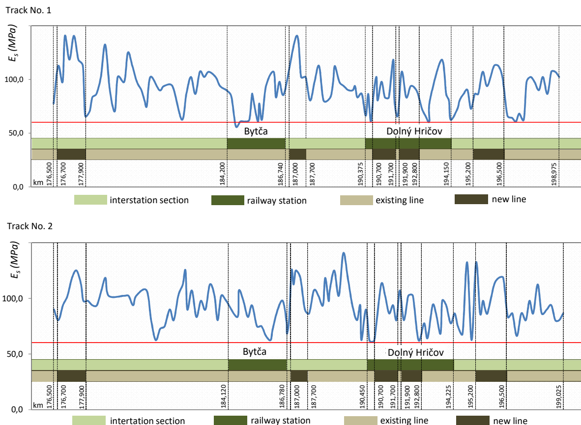
Figure 4. Graphic course of achieved values of deformation modulus of the formation of the railway subgrade surface.
